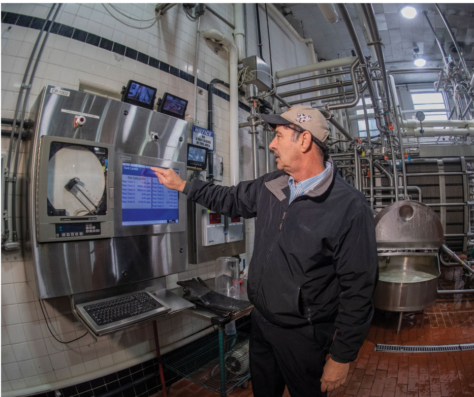
Brett Garner, director of operations, checks information on the computer-controlled pasteurization system.
